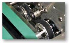
Customer Situation: GBR Systems Corp., a manufacturer of paper handling equipment, was using set screws to connect a high-speed drive pulley, running a Gates Polyflex JB belt, to a 3/8 in. shaft. The set screws would loosen during clutching and breaking at high RPMs, causing the machine to mal function and damage to the belt. Constant ly tightening the set screws resulted in loss of machine productivity and increased maintenance costs.
